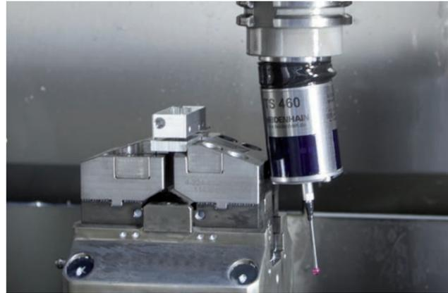
The collision protection adapter protects the spindle and touch probe
