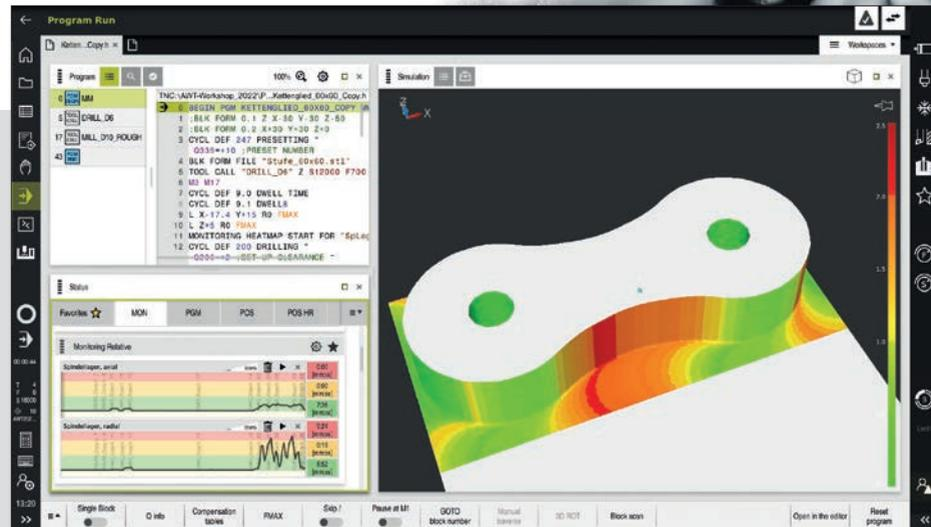
The Component Monitoring function of the TNC7 protects your valuable investment in a machine tool. It's a toolbox that allows machine manufacturers to implement extensive monitoring functions. During machining, this function can protect the spindle bearing from overloading, detect increased component wear in the drive chain, and more. It also delivers valuable data about actual loads acting on the machine, thus helping you evaluate process capability and benefit from predictive maintenance.
